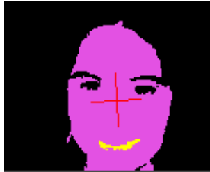
Fig. 7. The LAFTER system finds and tracks face and facial features at 30hz, feeding facial feature geometry for HMM expression recognition
