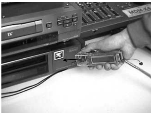
Fig. 4. The InfoStick programs a VCR to make a recording
