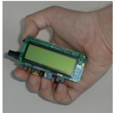
Fig. 1. The control appliance (a): A human selects a device in the environment (the controlled device (b)) with the help of a controlling device through a laser (1). After selection, commands are transmitted to the controlling device (2). A human chooses one of the displayed commands with the associated button at the Point & Select AIDE device (right figure).
