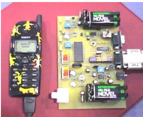
Fig. 5. Phone on a table together with the first prototypical sensor board. Phone in hand
