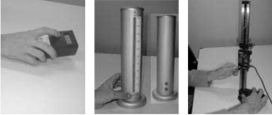
Fig. 10. Real height tools: Digit , a box with up-down buttons; Tower , a luminous scale with up-down buttons; Slider , a sliding-ruler with up-down handle and digital display (left to right).
